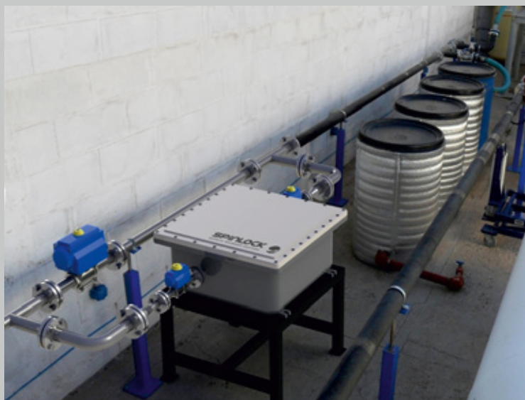
SLK-GOW testing in a multiphase Flow Loop
